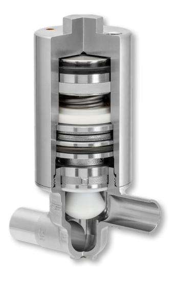
The GEMÜ F40 filling valve is perfect for filling liquid and viscous foodstuffs, cosmetics and pharmaceuticals. Simple, fast maintenance is possible thanks to the unique PD sealing concept with actuator fixing via a central thread and cartridge technology. Plus, the GEMÜ F40 is designed for multiple fast cycle duties, ensuring the filling machine is highly efficient.
