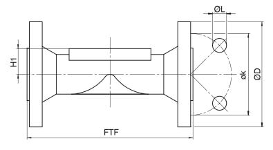
Connection type flange, length EN 558 (code 8)<sup>1)</sup>, forged material (code 40, 42)<sup>2)</sup>
