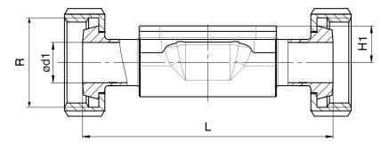
Connection type cone spigot DIN (code 6K)<sup>1)</sup>, forged material (code 40, 42)<sup>2)</sup>
