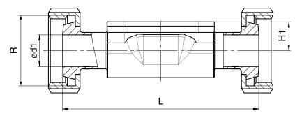
Connection type cone spigot DIN (code 6K)<sup>1)</sup>, forged material (code 40, 42)<sup>2)</sup>
