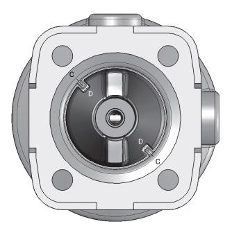
Place the compressor loosely on the actuator spindle, fit the recesses  ${\bf D}$  into the guides  ${\bf C}$ . It must be possible to move the compressor freely between the guides.
