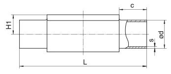
Connection type spigot DIN/EN/ISO (code 0, 16, 17, 18, 60)<sup>1)</sup>, forged material (code 40, 42, F4)<sup>2)</sup>
