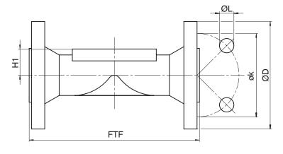
Connection type flange, length EN 558 (code 39), <sup>1)</sup> forged material (code 40, 42) <sup>2)</sup>
