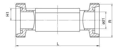
Connection type threaded spigot DIN (code 6)<sup>1)</sup>, forged material (code 40, 42)<sup>2)</sup>
