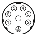
Plug assignment X2, S1/S2
