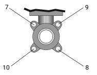
10. Tighten nuts **7 - 10** diagonally, holding them with a wrench.
