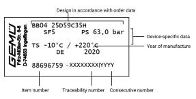
The month of manufacture is encoded in the traceability number and can be obtained from GEMÜ. The product was manufactured in Germany.
