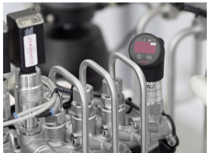
Pressure and temperature sensors
