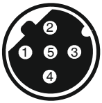
5-pin M12 built-in socket, D-coded
