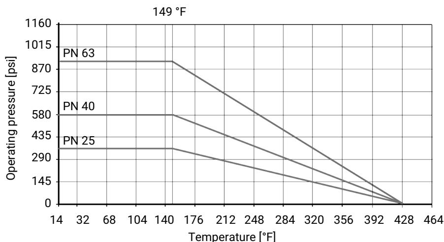
Pressure/temperature data in accordance with diagram refers to static operating conditions.
