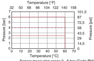
Sensor measuring range 0 - 6 bar (Code BH) Sensor measuring range 0 - 4 bar (Code BG) Sensor measuring range 0 - 2,5 bar (Code BF)
