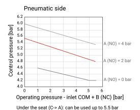
Operating pressure, inlet 1: Can be at B (NC) or COM + A (NO) Operating pressure, inlet 2: Can be at B (NC) or COM + A (NO)
