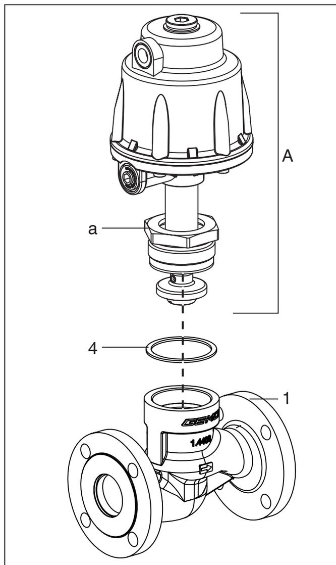
1. Mount actuator top (see chapter 7.1 "Installation of actuator top").
