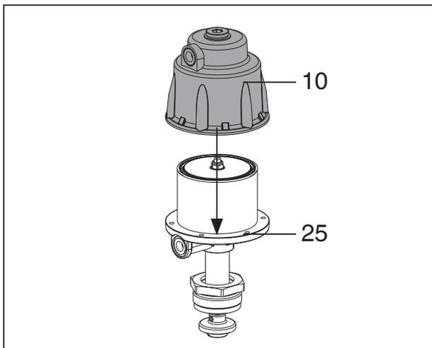
2. Ensure that the hole patterns of the actuator top **10** and actuator base **25** are aligned.
