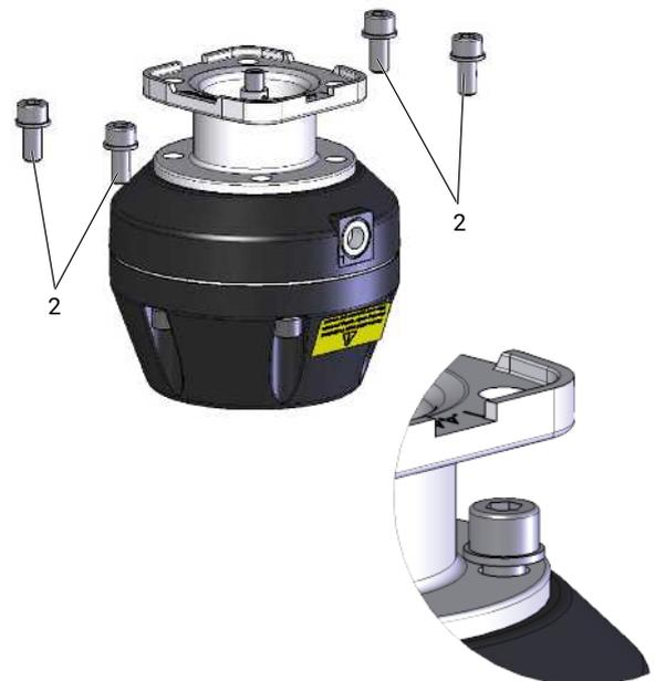
2. Assemble four cylindrical screws (2) with the integrated washer (screw-and-washer assembly).
