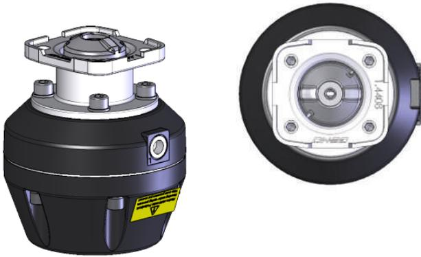
8. The actuator is now converted to the new QHD distance piece with the latest internally guided compressor.
