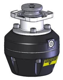
5. Once the new QHD distance piece has been centred, the four cylindrical screws must be screwed tight.
