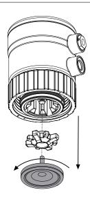
Remove the diaphragm from the actuator by turning it anticlockwise.
