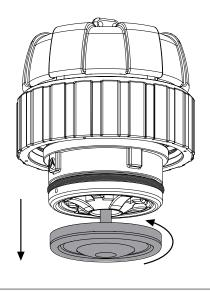
Unscrew the diaphragm from the operator by turning it anticlockwise.
