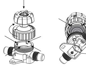
1. Press the operator onto the valve body.
