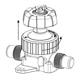
Carefully undo the central nut by hand and remove the operator from the valve body. 5
