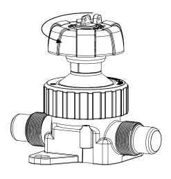
Open the valve fully by turning the handwheel anticlockwise.
