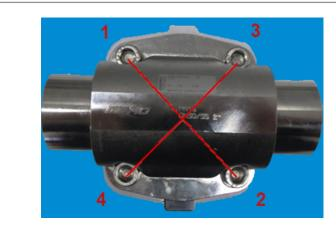
• Loosen the connecting bolts diagonally and lift the actuator off the valve body.
