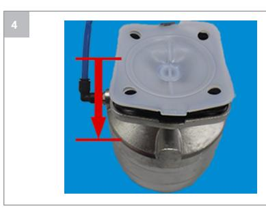
• Move the actuator to the open position.
