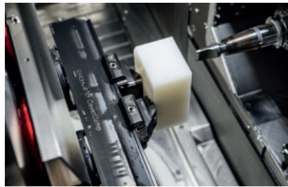
CNC manufacture and 100% testing of plastic block bodies
