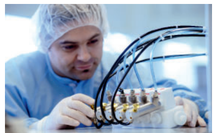
Assembly in the cleanroom and 100% testing (tightness etc.)
