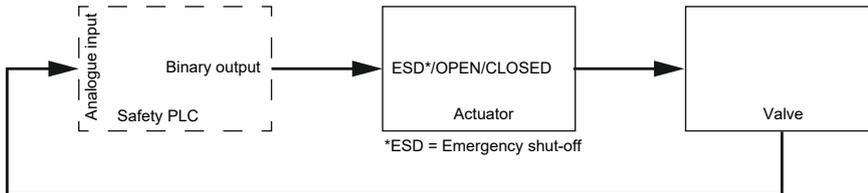
Fig. 1: Possible test set-up
